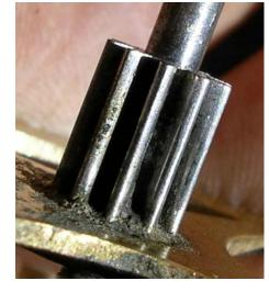
The clock had worn nice small (not always noticeable) steps into the pinion which fit the shape of the tooth engaging with the pinion and moves with wear in the holes (bushings). By installing new bushes which fit the pivots more precisely it changes the depth and brings the teeth of the wheel closer to the pinion therefore the previously perfectly fitting (worn) curves now JAM on each other.
