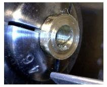
Step 6 - Turn the part around. The diameter of the top of the barrel arbor cup is 4.54mm, making the #46 collet the correct collet to hold it while working on the base. I would hesitate to use anything other than a #46 collet because other
