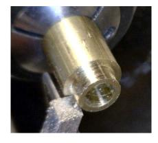
will see that there is a bevel. This bevel extends a little over half the distance to the outer edge, perhaps as much as 75%. Before starting the bevel, I verified that the area I cut away in Step 3 was indeed 1.75mm. With this height correct, I turned
