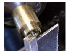
Step 5 - Parting off the cup: The work on the top part of the barrel arbor cup was now complete and the part needed to be cut off from the unused
