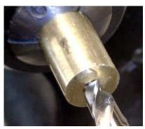
used to hold the drill bit if a collet holding tailstock is not available.
