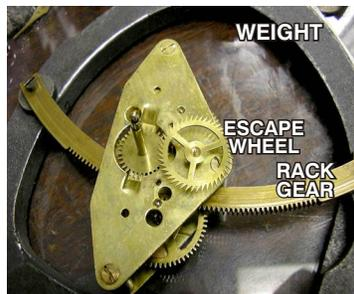
The rate is adjusted by a nut on the lower pendulum rod and the clock is wound once a day by pushing the lever on the side of the clock down which raises a half round weight inside the clock.
