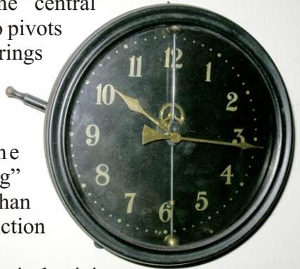
The disadvantage is that it is not very precise lining up with the escape wheel. So one cannot use this kind of bearing in a quality dead beat escapement where one degree makes a difference in the clock working or stopping. The larger arc Tic Tac escapement used in this case is more forgiving.
